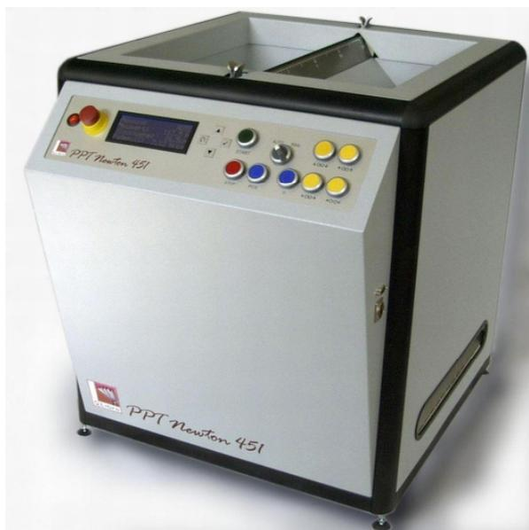
page. The measuring result is directly transferred into a computer via a serial interface. After each measurement the pulling and clamping mechanism automatically return into their original positions so that already after a few seconds the next measurement can be started.
